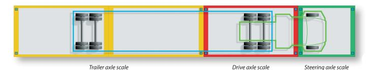
Avery Weigh-Tronix multi-platform scales can use any number and combination of 10', 12', 20', 23.5' or 25' standard length modules. Other sizes are available upon special request. Each section functions as an independent scale to provide accurate axle weights.
